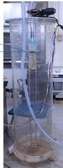
그림. 3 Schematic diagram of the Sequence Batch Reactor (SBR)
